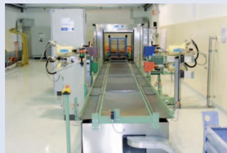
Release Measure- ment System for Packed Waste, Research Center Ispra (ITA)
